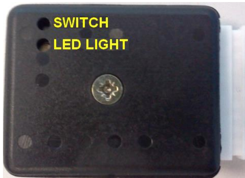
Figure 79 Adapter signaling led
